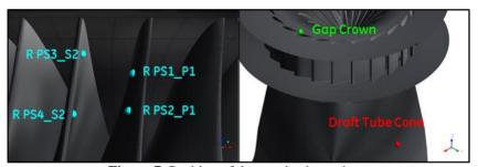
Figure 7: Position of the monitoring points
