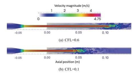
Fig. 2 Instantaneous velocity fields (medium grid) for two different values of the CFL numbers (top CFL = 0.6; bottom CFL = 0.1)—Re<sub>th</sub> = 3500
