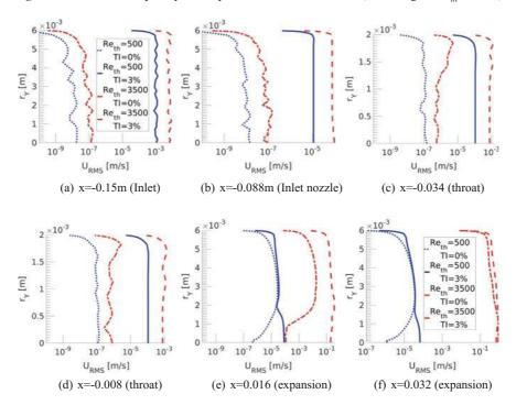
**Fig. 5** Radial profiles of the root-mean-square (RMS) velocity for the laminar ( $Re_{th} = 500$ ) and transitional ( $Re_{th} = 3500$ ) regimes at a variety of axial positions with and without TI (Medium grid)
