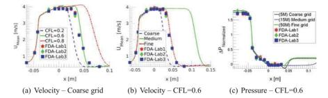
**Fig. 3** Longitudinal evolutions of the streamwise velocity (*left* and *middle* plots) and wall-pressure (relative to the pressure at x = 0 and normalized by the dynamic pressure at the throat—*right* plot) for a variety of temporal and spatial resolutions—Re<sub>th</sub> = 3500
