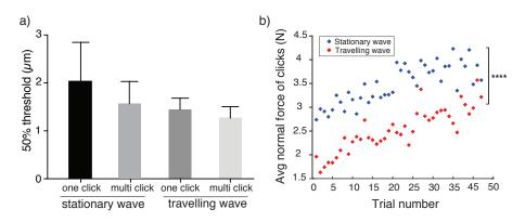
Fig. 5: a) Comparison of the perceptual thresholds between the multiple clicks and one click conditions for both actuation techniques. The boxplots and error bars show respectively the median values and the interquartile ranges. b) Scatter plot of the average peak normal force during pressing for a given trial number.
