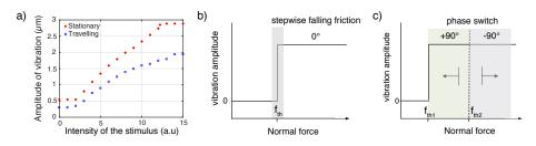
Fig. 2: a) The correspondance between the arbitrary intensity values and the amplitude of ultrasonic vibration. b) The keyclick actuated by the stationary wave was generated by a stepwise switch on of the ultrasonic vibration at a predefined threshold value of the normal force c) For the travelling wave, the stepwise increase in amplitude at  $f_{th1}$  is followed by a second normal force threshold  $f_{th2}$  at which the direction of the ultrasonic wave is reversed.
