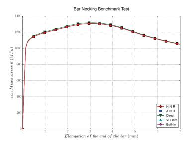
Figure 6: Von Mises stress  $\overline{\sigma}$  vs. displacement for the necking of a circular bar
