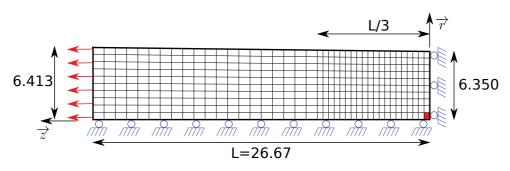
Figure 4: Numerical model for the necking of a circular bar
