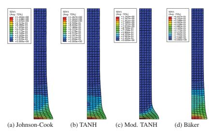
Figure 12: Equivalent plastic strain contour-plot of the Taylor specimen for the four constitutive models using the N-N-R VUMAT
