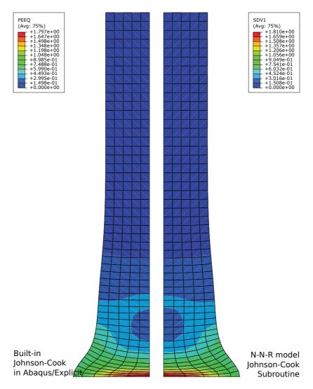
Figure 9: Equivalent plastic strain  $\overline{e}^p$  contourplot for the Taylor impact test
