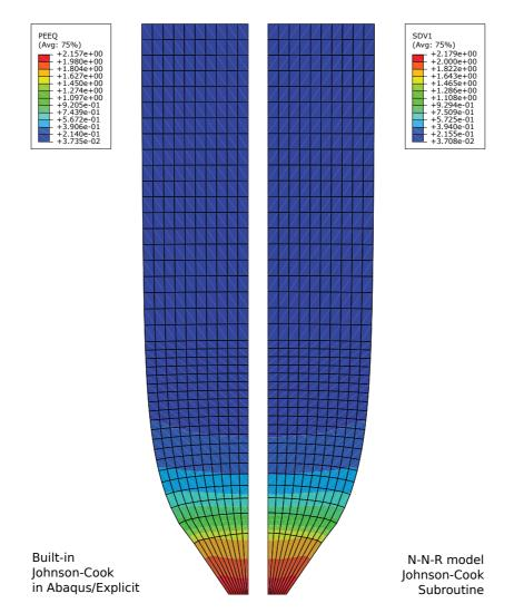
Figure 5: Equivalent plastic strain  $\overline{e}^p$  contourplot for the necking of a circular bar
