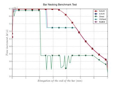
Figure 7: Time increment  $\Delta t$  vs. displacement for the necking of a circular bar
