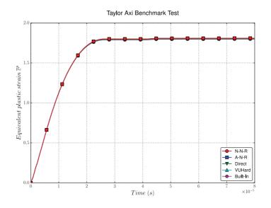
Figure 10: Equivalent plastic strain  $\overline{\varepsilon}^p$  vs. time for the Taylor impact test
