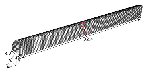
Figure 11: Model of the 3D Taylor impact test
