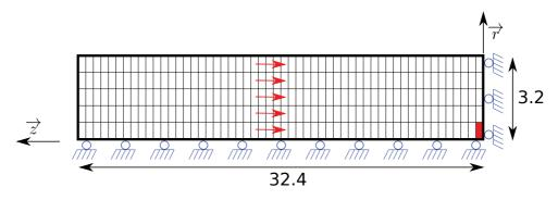
Figure 8: Model of the Taylor impact test
