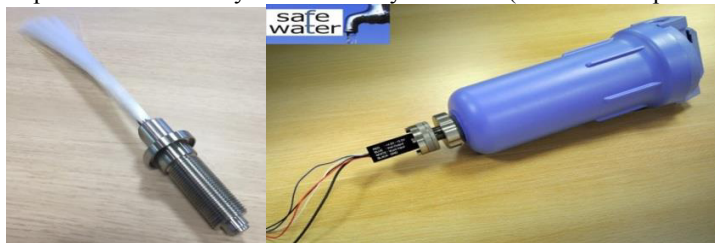
Fig. 4: left panel, scintillating optical fibre bundle. Right panel, scintillator bundle mounted with PMT in flow cell for water analyses.
