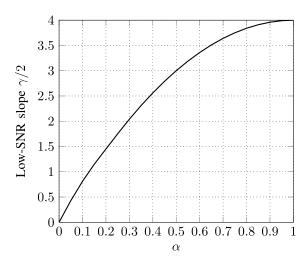
Fig. 3. The low-SNR asymptotic slope  $\gamma/2$ , see (50), is depicted as a function of  $\alpha \in (0, 1)$  for the two-LED MISO channel with gains  $h_1 = 3$  and  $h_2 = 1$  (the same channel as considered in Figure 2).
