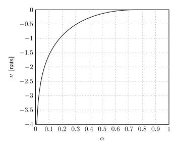
Fig. 2. The parameter  $\nu$ , see (34) and (49), is depicted as a function of  $\alpha \in (0,1)$  for the two-LED MISO channel with gains  $h_1=3$  and  $h_2=1$ . This represents the asymptotic capacity gap to the case with no average-power constraint, i.e., to  $\mathcal{C}_{\mathbf{h}^\mathsf{T},\sigma^2}(\mathcal{A},\mathcal{A})$ .
