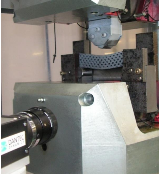
Fig. 11. Three-point bending test instrumented with an image correlation system
