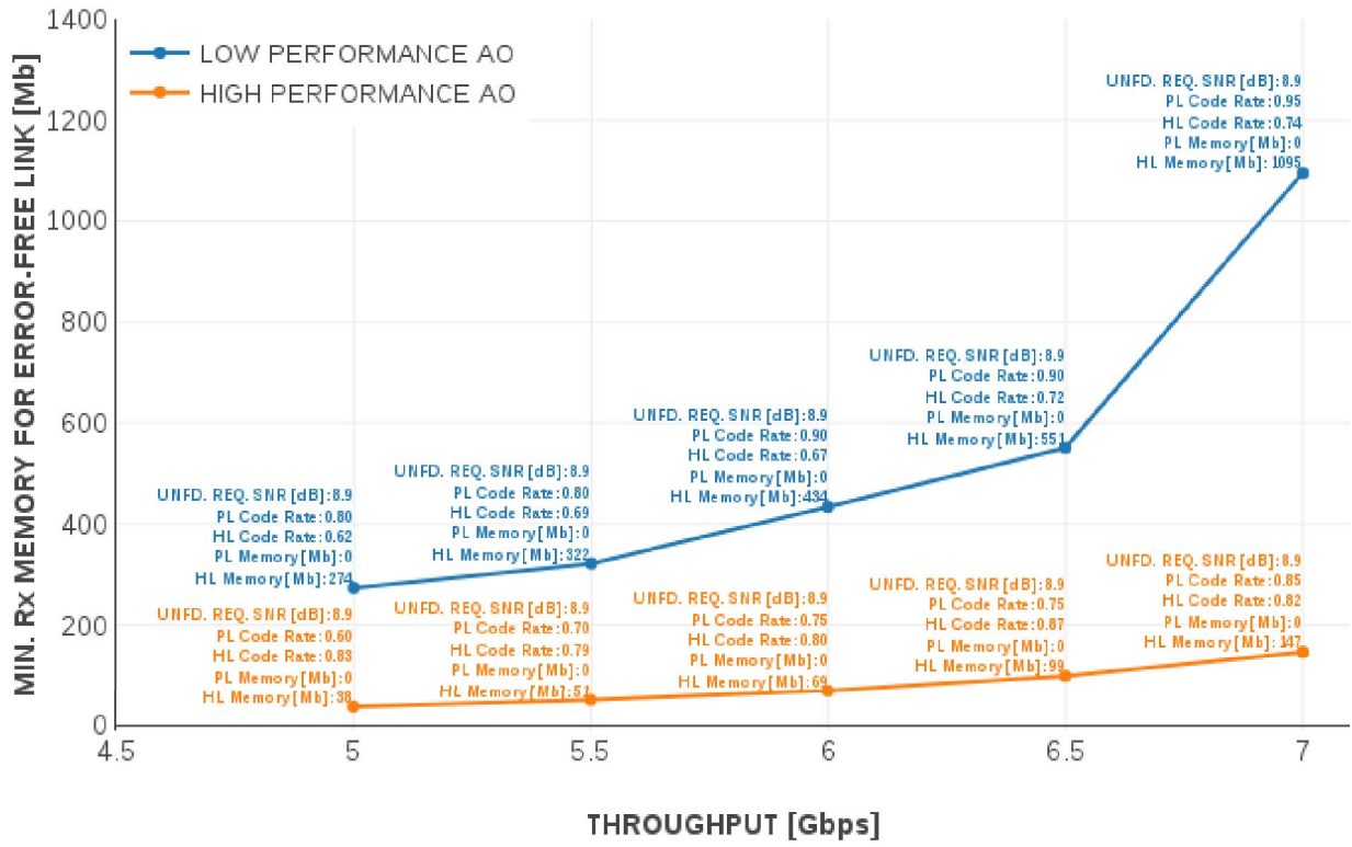
Fig. 2. Evolution of the minimum total memory of the receiver allowing an error-free transmission against the throughput.
