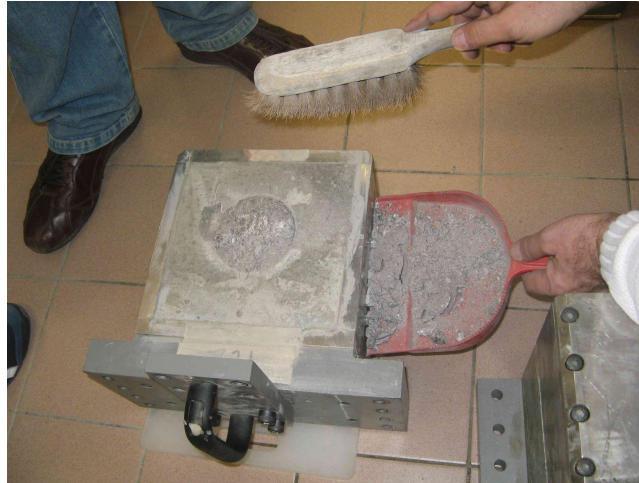
Figure 9: Infill material in one specimen of the tested rock joints
