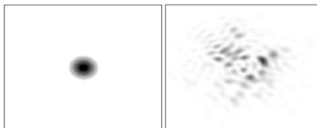
Figure 3 : Advantages of adaptive optics correction. Left: with correction. Right: without correction [14].
