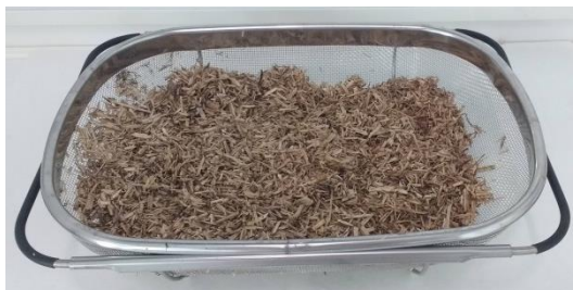
134 135 Figure 2. Sample of hemp shiv aged during two years in A_{Ext} conditions
