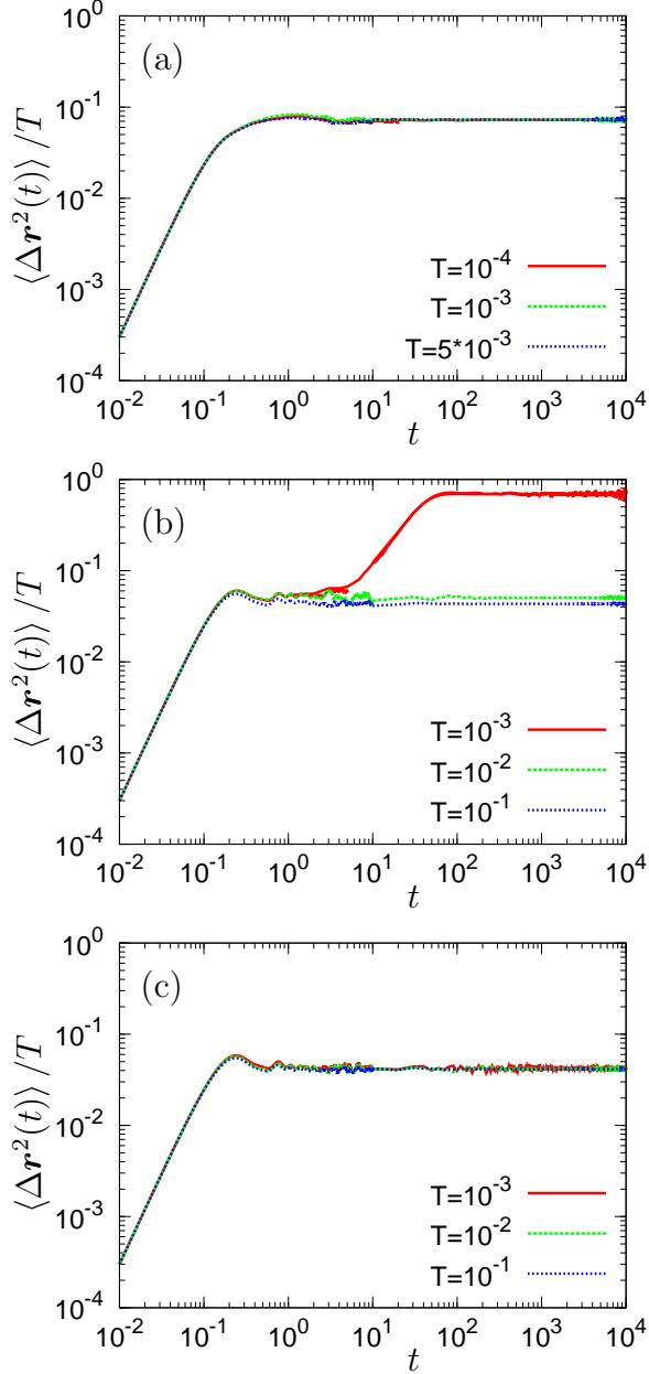
FIG. 7. Mean square displacement of particles,  $\langle \Delta \bar{r}^2(t) \rangle$  (Eq. (16)), is plotted as a function of time  $t$ , for (a) glass 1, (b) crystal 1, and (c) crystal 2. The value of  $\langle \Delta \bar{r}^2(t) \rangle$  is normalized by the temperature  $T$ . Different lines represent three temperatures as indicated in the key. In the harmonic regime values of  $\langle \Delta \bar{r}^2(t) \rangle / T$  for different  $T$  collapse onto a single curve.
