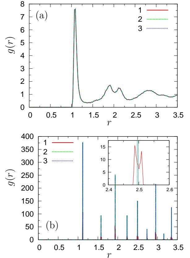
FIG. 2. The RDF  $g(r)$  in the energy minimum state ( $T = 0$ ) for (a) glasses and (b) crystals. The values for three types of truncated potentials, 1 (red solid line), 2 (green dashed line), and 3 (blue dotted line), are presented. The inset to (b) is a close-up around  $r = 2.5$ .
