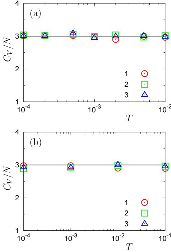
FIG. 13. The temperature,  $T$ , dependence of the specific heat per particle,  $C_V/N$  (see Eq. (23)), for (a) glasses and (b) crystals. If thermal vibrations are harmonic,  $C_V/N = 3$  - shown as the horizontal solid line.
