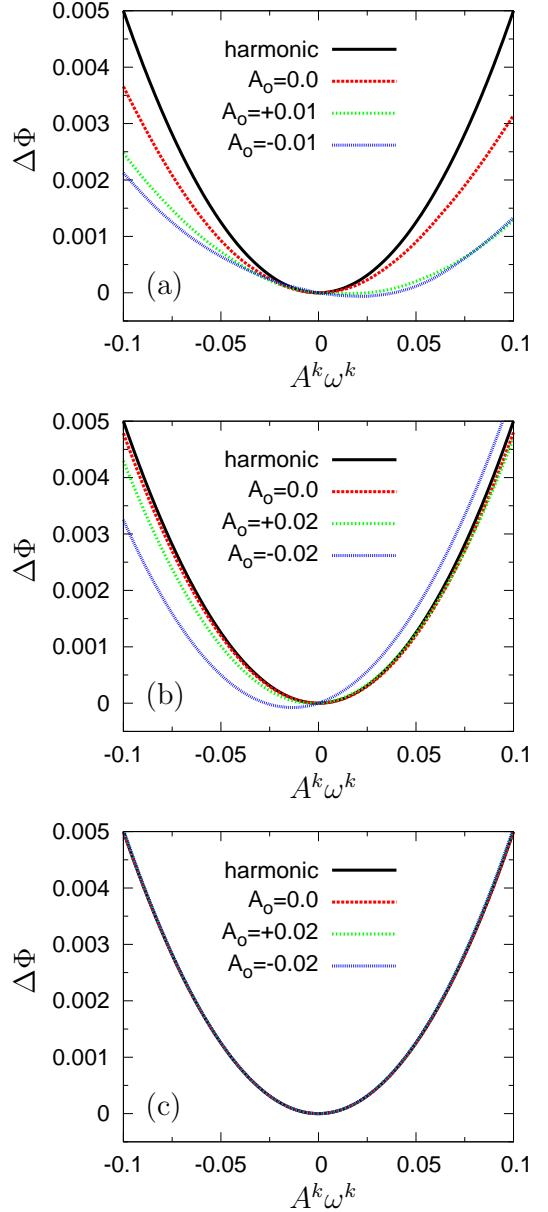
FIG. 9. The potential energy landscape,  $\Delta\Phi(A^k, A_o)$ , along (a) low  $\omega^k = 2.19$  and (b) high  $\omega^k = 8.91$  modes in crystal 1, and (c) low  $\omega^k = 2.12$  mode in crystal 2. See also the caption of Fig. 8.
