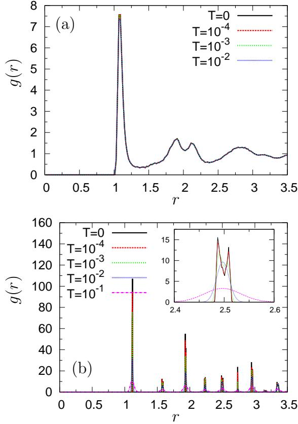
FIG. 10. The RDF  $g(r)$  for (a) glass 1 and (b) crystal 1 at zero,  $T = 0$ , and finite,  $T > 0$ , temperatures. The inset to (b) is a close-up around  $r = r_c = 2.5$ . The data at  $T = 0$  are same as those presented in Fig. 2.
