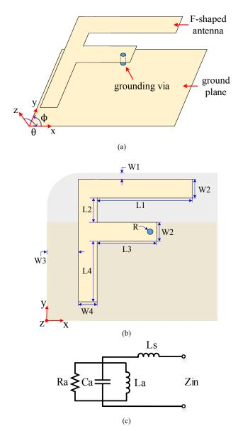
Figure 2. Geometries and an equivalent circuit of the proposed F-shaped antenna: (a) 3-D view with substrate board removed; (b) Top view; (c) The equivalent circuit of the antenna.
