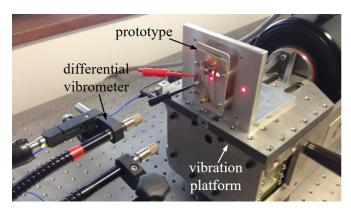
Figure 6. The measurement setup to test the mechanical resonator of the hybrid power harvester.
