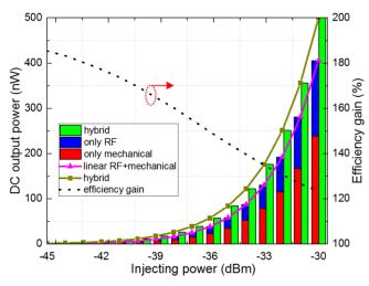
Figure 4. Comparisons of DC output power rectified from hybrid and separate harvesting modes together with efficiency gain performance when both RF and mechanical powers injecting into diode are swept from -45 to -30 dBm.
