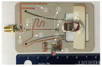
Figure 5. Photo of the experimental prototype of the proposed hybrid microwave and mechanical power harvester.
