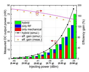
Figure 11. Measured DC output power from separate and hybrid modes together with simulated DC output from the hybrid mode. Comparison of measured and simulated efficiency gain is also demonstrated.
