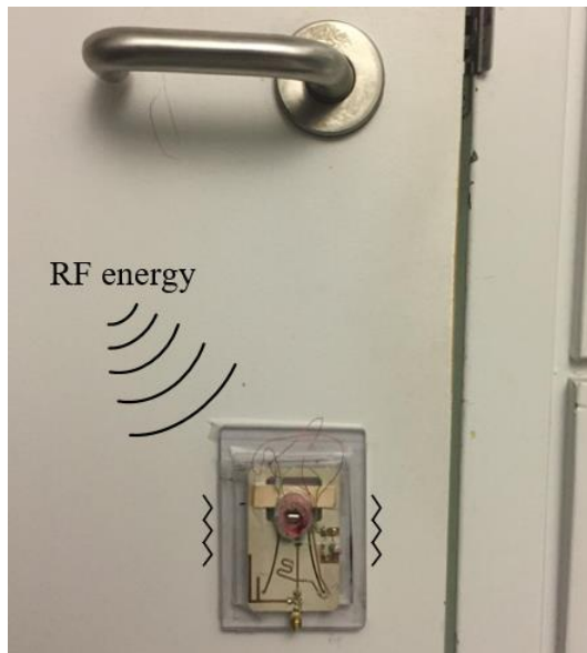
Figure 12. Implementation of proposed hybrid energy harvester on a door frame, which takes advantage of the vibration just after the door closes.
