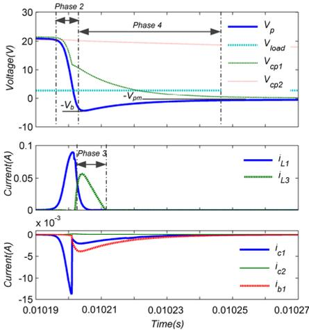
Fig. 5. Zoomed waveforms around the inversion instant.
