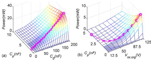
Fig. 11 (a) Power versus  $C_0$  and  $C_p$  with  $V_{oc,org}$  constant as 37.5V; (b)  $V_{load}$  versus  $u_M$  and  $C_p$  with  $C_0$  constant as 13.75nF.
