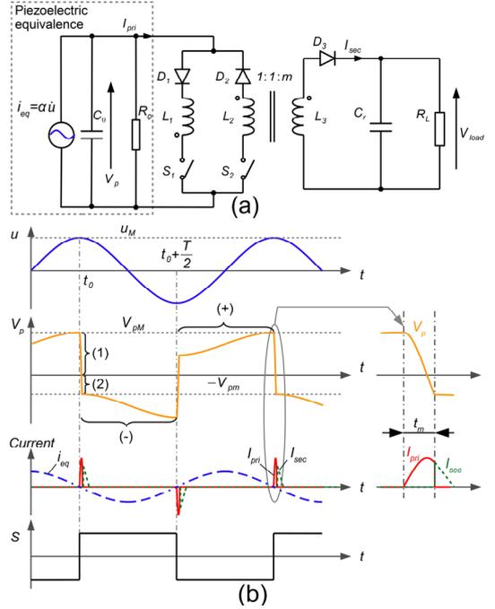
Fig. 1. (a) OSECE approach; (b) Typical waveforms.
