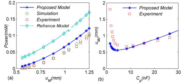
Fig. 9 (a) Power versus displacement magnitude  $u_M$ ; (a) Critical starting displacement  $u_{Mc}$  versus  $C_p$ .
