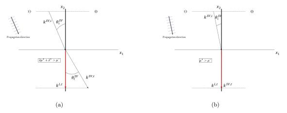
Figure 8: Possible manifestations of Stoneley waves at a Cauchy/Cauchy interface for L and SV transmitted modes in the case of incident SV wave. The vectors in black represent propagative modes, while the vectors in red represent modes which propagate along the surface only (Stoneley modes).
