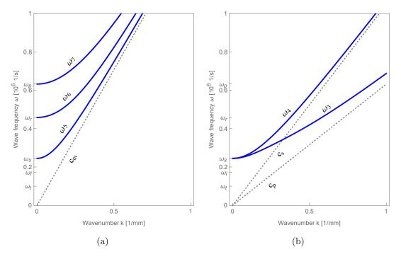
Figure 24: (a) Three distinct modes have distinct cut-off frequencies but a common asymptote with slope  $c_m$ , (b) Two distinct modes have the same cut-off frequencies but asymptotes with different slopes  $c_f$  and  $c_p$ .
