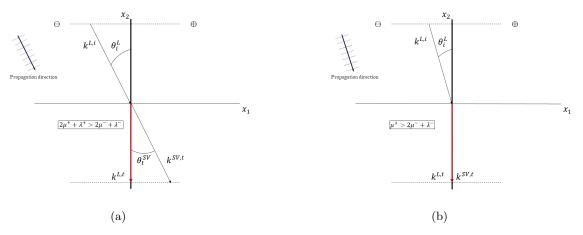
Figure 7: Possible manifestations of Stoneley waves at a Cauchy/Cauchy interface for L and SV transmitted modes in the case of incident L wave. The vectors in black represent propagative modes, while the vectors in red represent modes which propagate along the surface only (Stoneley modes).
