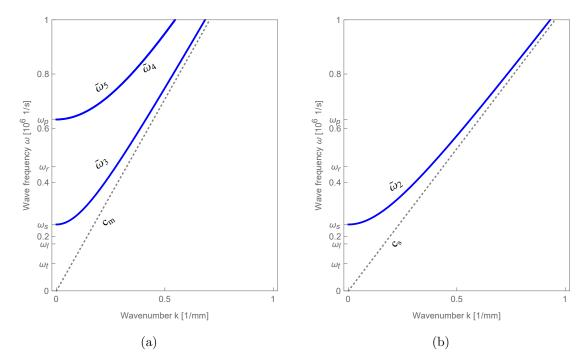
Figure 26: (a) First mode with cut-off frequency  $\omega_p$  and second and third modes which overlap for large values of  $|\tilde{k}|$ , all have the same asymptote  $c_m$ , (b) The fourth mode has an asymptote with slope  $c_f$ .
