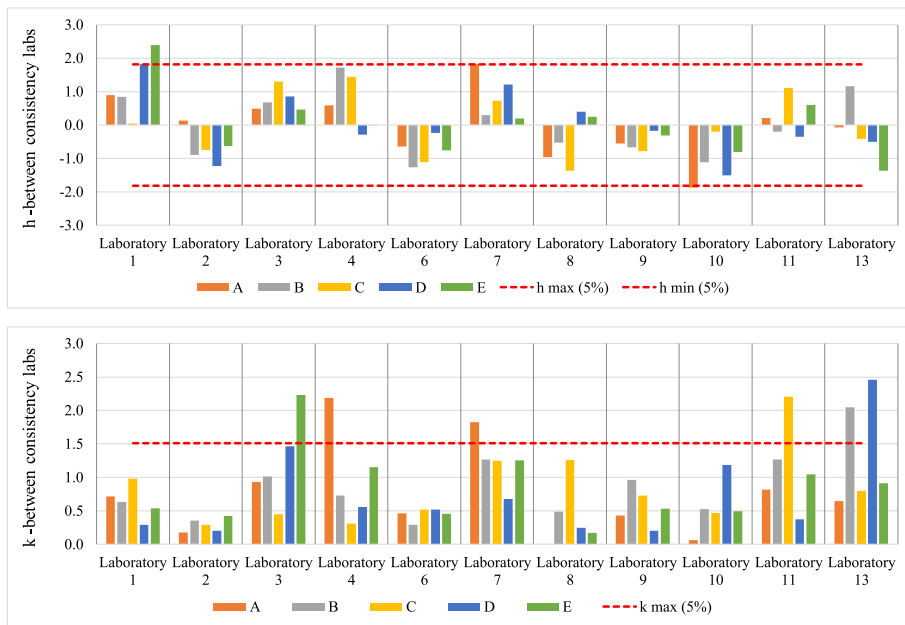
Fig. 15. The values of h and k Mandel's tests for the loss factor.
