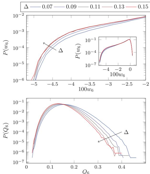
FIG. 7. Effect of polydispersity on local structures at constant pressure ( $\beta p\sigma^3 = 23$ ): (top) detail of the distribution of  $w_6$  (full distribution in inset) showing a small increase in the icosahedra population saturating around 10%; (bottom) distribution of  $Q_6$  showing a marked decrease in the crystallinity with polydispersity.
