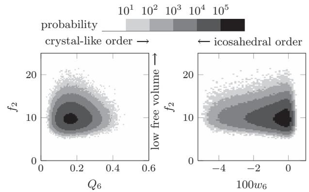
FIG. 3. Correlation between two-body and many-body parameters. Probability distribution functions in the  $f_2$ - $Q_6$  map (left) and in the  $f_2$ - $w_6$  map (right) for a metastable fluid with polydispersity  $\Delta = 7\%$  and pressure  $\beta p \sigma^3 = 23$ . There is no linear correlation between the parameters, meaning that high values of  $Q_6$  (the crystalline regions) or low values of  $w_6$  (the icosahedral regions) are not extremum values of  $f_2$ .
