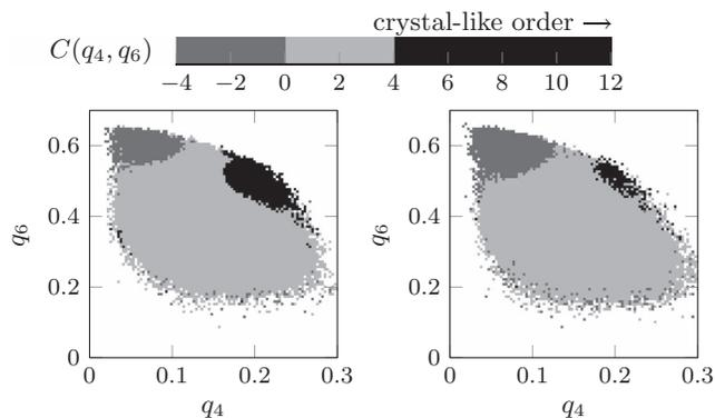
FIG. 8. Average crystallinity order parameter projected on the  $q_4$ - $q_6$  plane for the metastable fluid at  $\beta p\sigma^3 = 23$  at  $\Delta = 7\%$  (left) and  $\Delta = 15\%$  (right). Icosahedra appear in the top-left corner of each plot (in dark gray) and perfect fcc crystals would be in the top-right corner with  $C = 12$  (in black).
