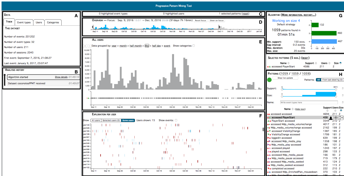
Figure 1: The main interface of PPMT: (A) Information about the dataset, (B) history of the analyst’s actions, (G) information about the state of the pattern mining algorithm and (H) discovered frequent patterns. Temporal visualization views present information from the dataset and the selected patterns: (D) overview of the data, (E) events and pattern occurrences, (F) user sessions and pattern occurrences. Analysts can select event types and users to highlight them in the temporal views. Selecting patterns adds their occurrences to the views. (C) A summary of the selections is always available.
