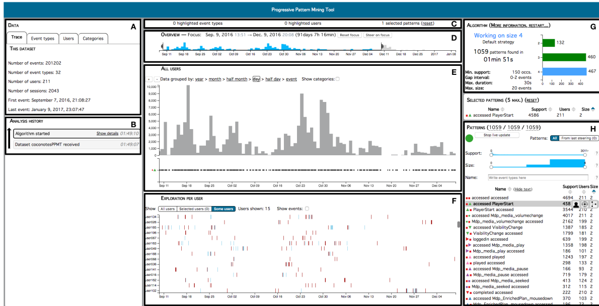
Figure 1: The main interface of PPMT: (A) Information about the dataset, (B) history of the analyst’s actions, (G) information about the state of the pattern mining algorithm and (H) discovered frequent patterns. Visualizations present information from the dataset and the selected patterns: (D) overview of the data, (E) events and pattern occurrences, (F) user sessions and pattern occurrences. Analysts can select event types and users to highlight them in the visualizations. Selecting patterns add their occurrences to the visualizations. (C) A summary of the selections is always available.
