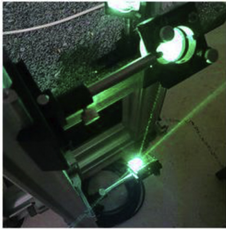
Fig. 7. Laser impact test stand.
