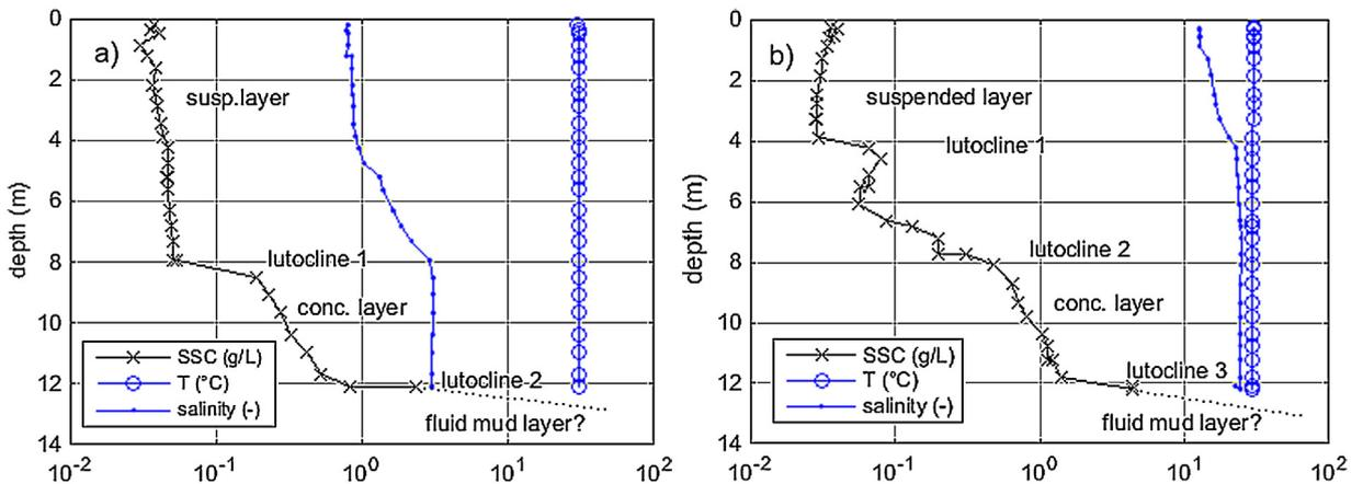
Fig. 2. Vertical stratification of the water column measured at a) transect T1 on 11<sup>th</sup> December 2015 at 17:30 local time; b) transect T3 on 10 December 2015 at 17:07 local time.
