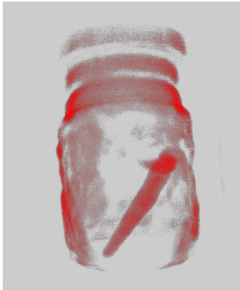
FIG. 6. Projection of the reconstructed pillbox where every low-attenuation coefficient voxels have been made transparent.
