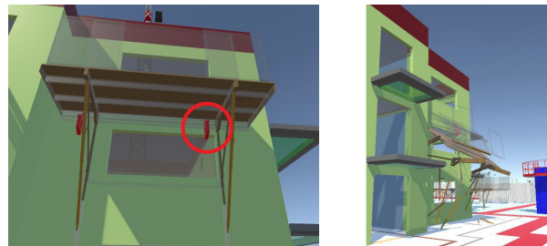
Fig. 5. Example of misplacement of fixings of PTE platform in the virtual environment. On the left, one fixing is misplaced (above an opening). On the right, this is what the trainee will see if he walks away from the PTE platform if he does not signal error.
