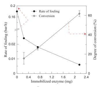
Fig. 6. Effect of amount of Enz<sup>SP</sup> deposited per membrane area on the rate of fouling and degree of conversion. The transmembrane flux was fixed at  $15 \text{ L/m}^2$  h, temperature 40 °C and pH 4.5.
