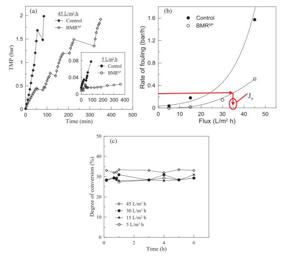
Fig. 3. a) The TMP profile of BMR<sup>SP</sup> and a parallel control system at 5 and 45 L/m<sup>2</sup> h, b) relation between flux and c) degree of conversion at each flux values, at 0.3 g/L feed concentration, 40 °C and pH 4.5 (results are within 5.2% experimental error).
