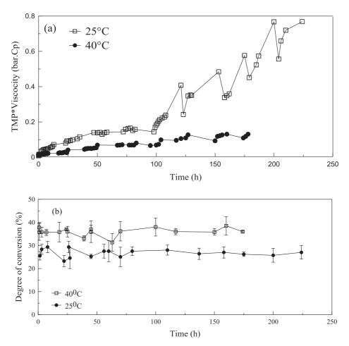
Fig. 7. Operational stability of BMR<sup>SP</sup> operated at 0.3 g/L, 5 L/m<sup>2</sup> h and 3 g/m<sup>2</sup> (2 µm) Enz<sup>SP</sup>, constant magnetic field, operated continuously for two weeks: a) TMP trend at 25 °C and 40 °C, b) Degree of conversion at 25 °C and 40 °C.
