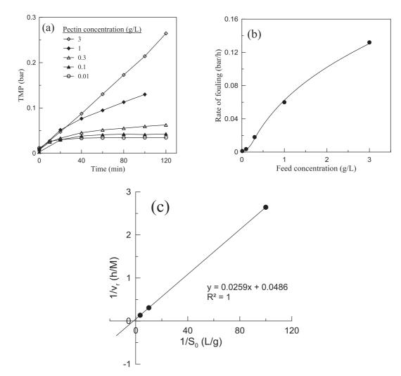
Fig. 5. Relation between a) feed concentration and TMP, and b) feed concentration, degree of conversion, rate of fouling and amount of GalA produced at 15 L/m<sup>2</sup> h, 40 °C and pH 4.5. c) Lineweaver-Burk plot.
