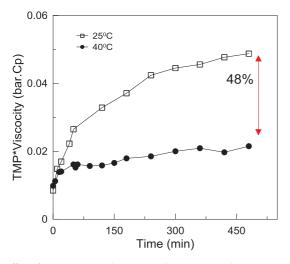
**Fig. 4.** Effect of temperature on the transmembrane pressure development: 0.3 g/L feed concentration,  $15 \text{ L/m}^2 \text{ h}$  flux, the TMP in the y-axis is normalized by the viscosity of the feed solution at 25 °C and 40 °C.
