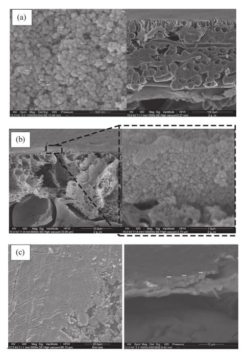
**Fig. 2.** a): Surface and b): cross-sectional SEM image of the biocatalytic layer containing 4.8 mg of Enz<sup>SP</sup>, revealing an average bed thickness of 2–3 µm on the top of the membrane active layer. c): Surface and cross-sectional SEM image of fouled membrane with a total thickness of foulant plus nanoparticle corresponding to 4 µm after continuous filtration of 0.3 g/L pectin for 6 h on a dynamic layer containing 4.8 mg of Enz<sup>SP</sup>.
