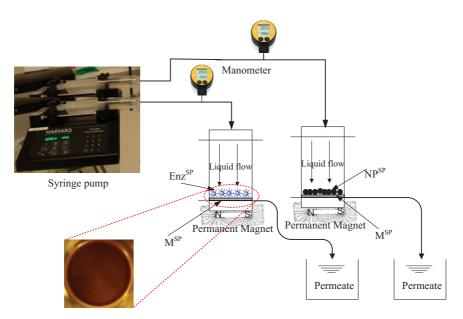
Fig. 1. Schematic illustration of the filtration set-up containing a syringe pump with two heads, two syringes each with 100 mL capacities, dead end filtration cell containing dynamic layer of pectinase activated magnetic nanoparticles (Enz<sup>SP</sup>), parallel control filtration cell containing dynamic layer of neutral magnetic nanoparticles (NP<sup>SP</sup>) and two parallel permeate tanks and digital manometers.
