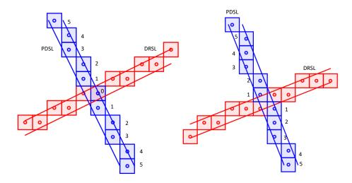
**Fig. 2.** The image of each point is the mirror image in the perpendicular line according to the digital reflection straight line. The image of a point numbered i is the opposite point numbered i. The point numbered 0 is its own image.
