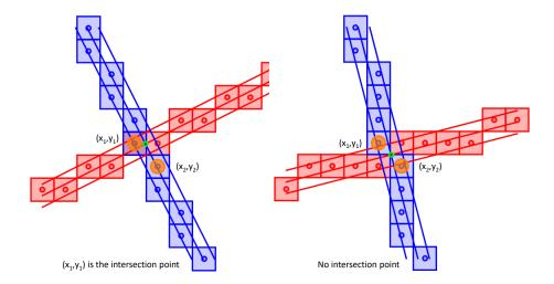
**Fig. 3.** The green point represents the intersection point between the continuous reflection line and the continuous perpendicular line. The orange disks mark the two candidate points for the digital intersection. On the left  $(x_1, y_1)$  is the digital intersection point between the DRSL and the PDSL. On the right there is no digital intersection point.
