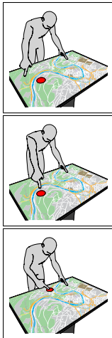
Figure 2: From top to bottom. a) A red anchor is added to the screen. b) The index of the right hand is linked to the anchor. c) The anchor is moved and the arm follows.
