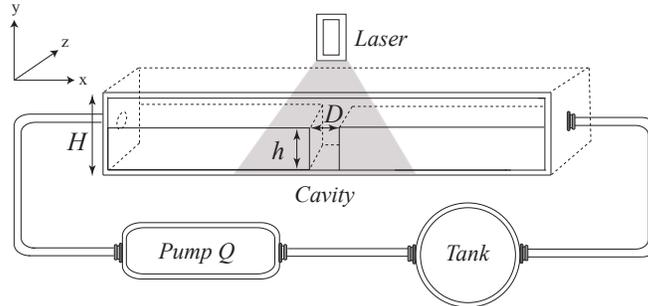
Figure 1: Schematic representation of the experimental setup. Dimensions of the cell are: length 30 cm, height  $H = 6.5$  cm, width 8 cm. The cavity of depth  $h$  and length  $D$  is located in the middle of the cell. Flow rate  $Q$  is controlled by a pump in a closed-loop circuit. A vertical laser sheet illuminates the cavity area at half-width of the cell.
