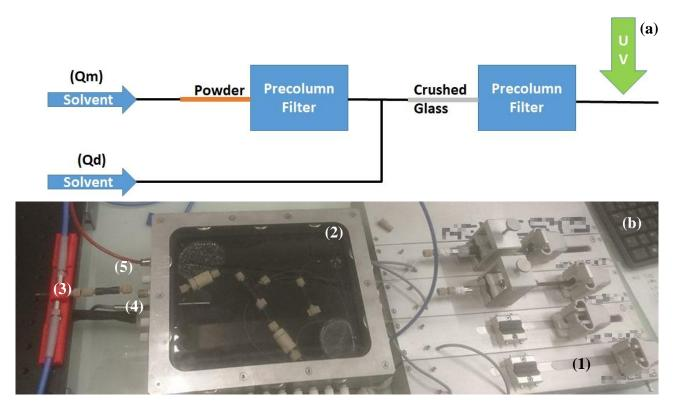
Figure 3. (a) Scheme and (b) photograph of the home-made microfluidics set-up: (1) syringe pump, (2) temperature controlled incubator, (3) UV cell, (4) temperature probe and (5) outside loop insuring solution thermal equilibrium to room temperature.
