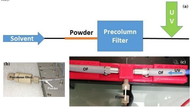
Figure 1. (a) Scheme of the dissolution set-up, (b) powder placed in a 1 mm inner diameter (ID) tube connected to a precolumn filter and, (c) UV cell, optical fiber (OF) light source (UV) from the right to UV spectrophotomer (left).
