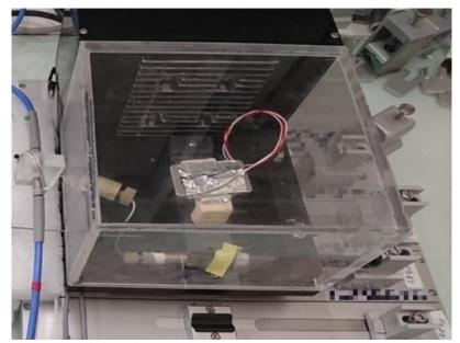
Figure S1. Temperature controlled incubator.
