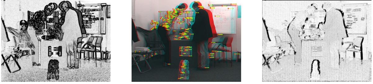
(a) SSIM map before transform (b) optimized matched feature point pairs (c) SSIM map after transform
