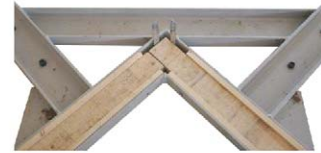
(c) Mudsill locked by a wooden wedge
