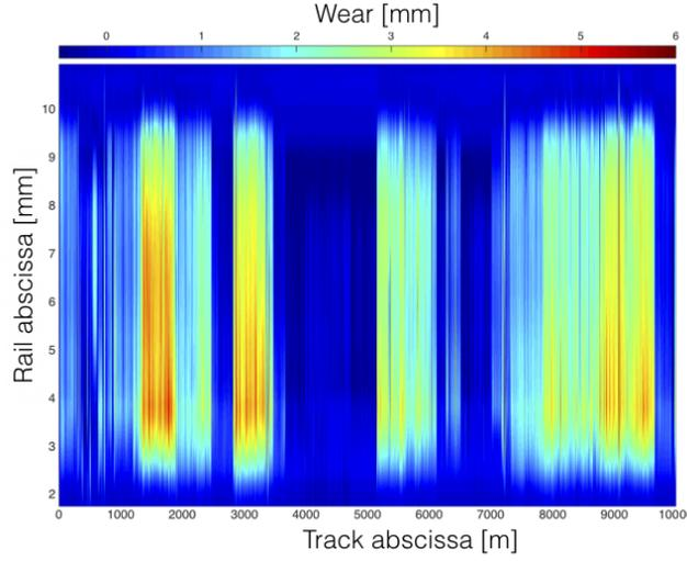
FIGURE 2 – Example of rail wear measurement.
