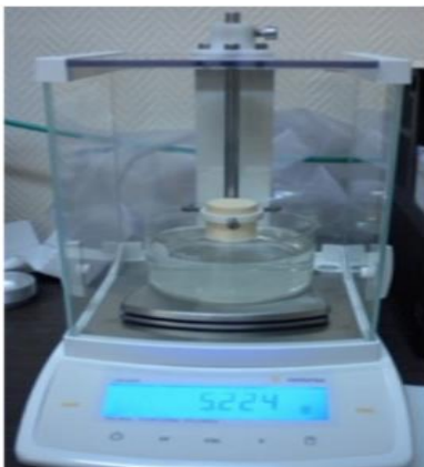
Figure 4- The non-reactive impregnation test
