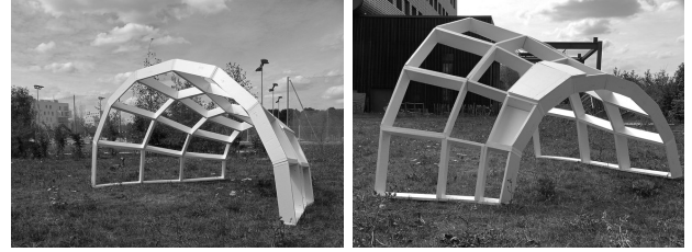
Figure 17: A model of a canal surface with planar quadrangles used for bracing.
