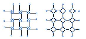
Figure 18: Nexorade pattern viewed as mesh patterns: topological equivalence between the alternated quad nexorade pattern and the truncated square pattern.
