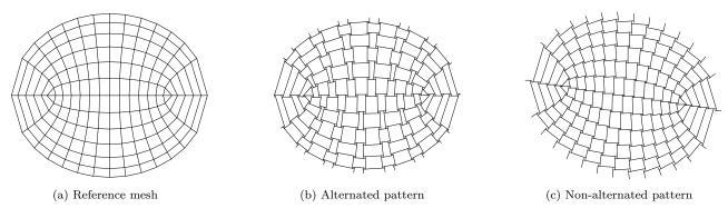
Figure 14: Comparison of the alternate and non-alternate translations for the fitting of an ellipsoid ( $\alpha = 0.1, \lambda = 0.8$ ).
