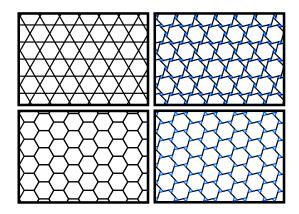
Figure 4: Nexorades (right) obtained from mesh patterns (left)
