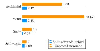
Figure 24: Maximal displacements (mm) for different load cases.
