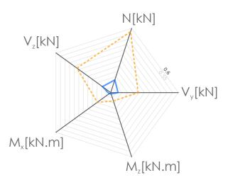
Figure 23: Average amplitude of forces and moment in connections for shell-nexorade hybrid (thick blue) and nexorade without panels (dotted orange).
