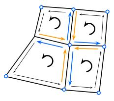
Figure 9: The half-edge data structure on a quadrangular mesh: ingoing (in orange) and outgoing (in blue) half-edges for the central node.
