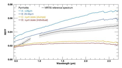
Fig. 7 - Spectra of ground pyrrhotite. The spectra A and B correspond to hand-ground and sieved samples. The sample C and D underwent 180 min colloidal grinding with the planetary grinder and contain only grains < 25  $\mu m$ . The sample C contains clumps because it has not been hand mixed after drying unlike the sample of the spectrum D.
