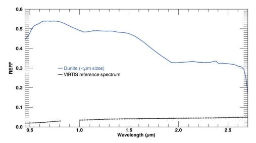
$\textbf{Fig. 6} - \text{Dunite spectrum compared to VIRTIS reference spectrum. The sample of dunite is sieved} < 25~\mu\text{m} \text{ after a 180 min colloidal grinding in the planetary grinder.}$
