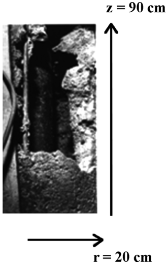
Figure 5. Trapping experimental results of NaH on cold walls.
