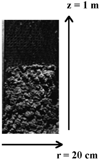
Figure 6. Trapping experimental results of Na 2 O on wire mesh.
