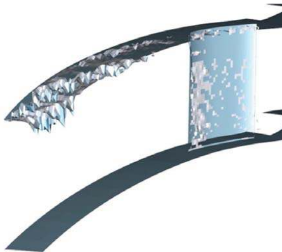
Fig. 20 approximation of the accreted ice thickness in the EGV stage for the reference case.
