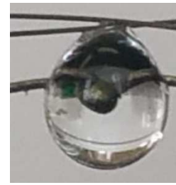
Figure 3: 400 \mu\text{m} thermocouple in suspended droplet
