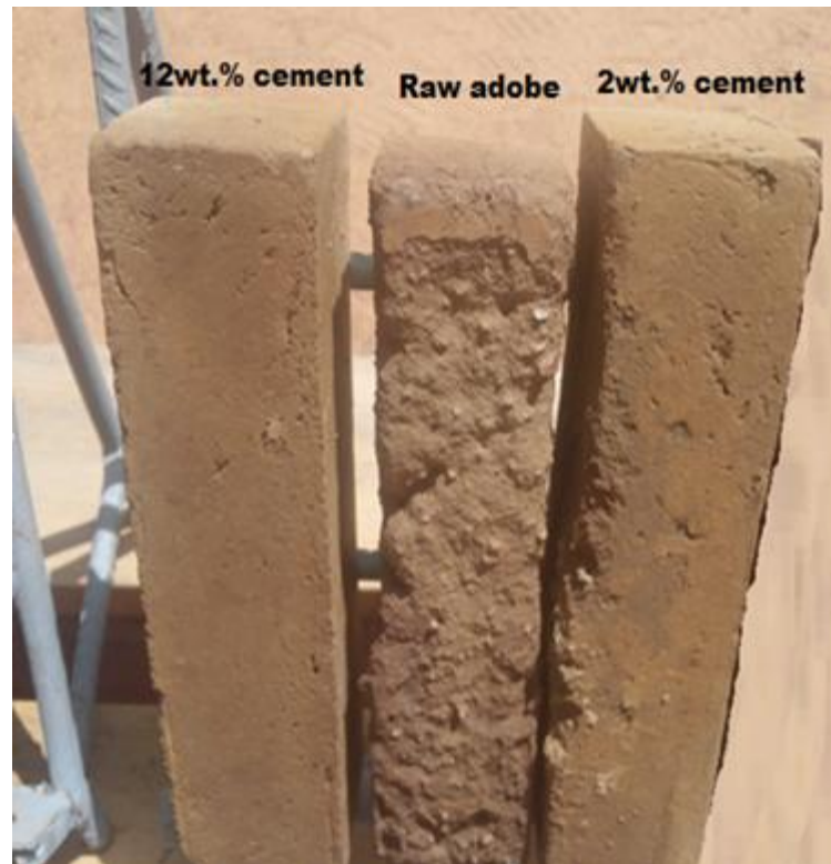
Figure 17: Images of adobes after spray test
