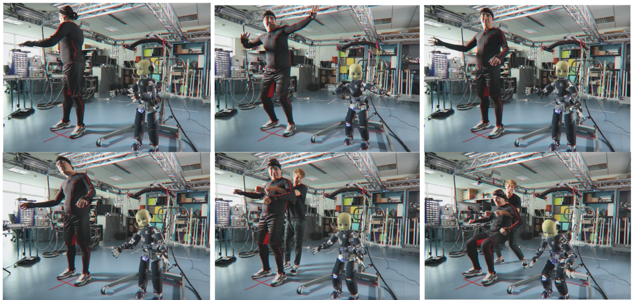
Fig. 10: Snapshots from the teleoperation experiment. Remarkably, the robot does not fall when the human operator falls back (frame on the bottom-right).
