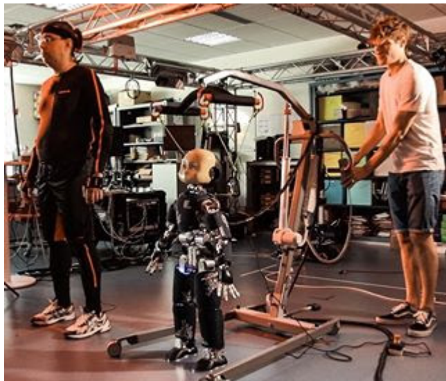
Fig. 1: Teleoperation of the iCub robot by an operator equipped with the XSens motion capture suit.
