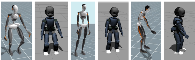
Fig. 7: Snapshots of the teleoperated simulated robot and of the Xsens skeleton while performing a squat motion, a hip roll exaggerate motion and a grasping motion during the teleoperation.
