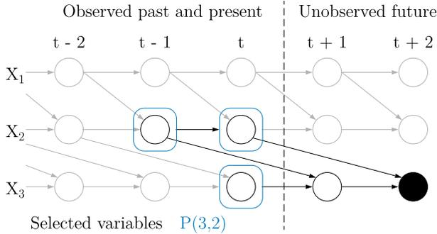
Fig. 1: Selection of relevant variables from a TiGraMITe graph. The predicted variable is  $X_3(t+2)$  (black node). Its parents are  $X_2(t)$  and  $X_3(t+1)$ . Because  $X_3(t+1)$  is still in the unobserved future, it cannot be used to produce a forecast. We have to go back to its own parents,  $X_2(t-1)$  and  $X_3(t)$ , which are already known at time  $t$ . Therefore, we can include them in the set of selected variables  $P(3,2)$  – (in blue). This figure is adapted from Fig.1 in [24].
