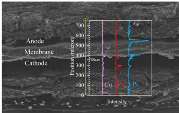
Fig. 3. Representative SEM micrograph (1,400 x magnification) of the cross-section of  $\text{TiO}_2(0.06\text{AR})\text{-PtCo/C}$  catalyst, and (inset) the EDX-derived line scan of Pt, Co and Ti particles.
