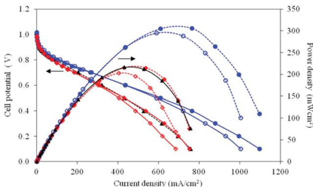
Fig. 4. Current density-potential curves of a single  $\text{H}_2/\text{O}_2$  PEM fuel cell with the as-prepared PtCo/C catalyst in the ( $\blacktriangle$ ) absence of  $\text{TiO}_2$ , and in the presence of ( $\bullet$ ,  $\circ$ )  $\text{TiO}_2(\text{R})$  or ( $\blacklozenge$ ,  $\blacklozenge$ )  $\text{TiO}_2(\text{AR})$  at a loading of ( $\bullet$ ,  $\blacklozenge$ ) 0.06 and ( $\circ$ ,  $\blacklozenge$ ) 0.15  $\text{mg}/\text{cm}^2$ .
