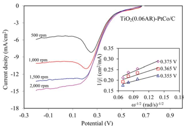
Fig. 7. Example of voltammogram for the ORR of  $\text{TiO}_2$ -PtCo/C catalyst and (insert) the Koutecky-Levich plots.
