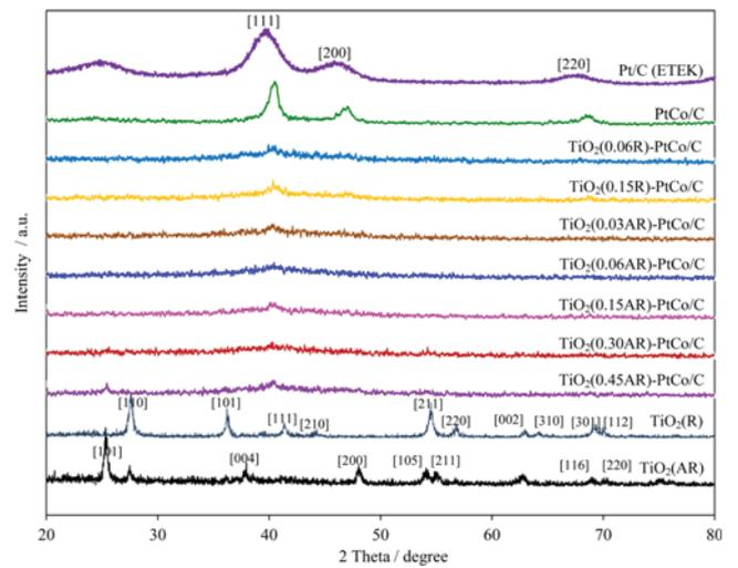
Fig. 1. Representative XRD patterns of the commercial Pt/C (E-TEK) and the as-prepared PtCo/C catalysts in the absence or presence of TiO<sub>2</sub>(R) or TiO<sub>2</sub>(AR) at different loadings.
