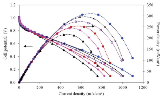
Fig. 5. Current density-potential curves of a single  $\text{H}_2/\text{O}_2$  PEM fuel cell of the as-prepared  $\text{TiO}_2(\text{AR})\text{-PtCo/C}$  catalyst at  $\text{TiO}_2$  loadings of ( $\blacktriangle$ ) 0.0, ( $\blacksquare$ ) 0.03, ( $\bullet$ ) 0.06, ( $\times$ ) 0.15, ( $\circ$ ) 0.30 and ( $\blacklozenge$ ) 0.45  $\text{mg}/\text{cm}^2$ .
