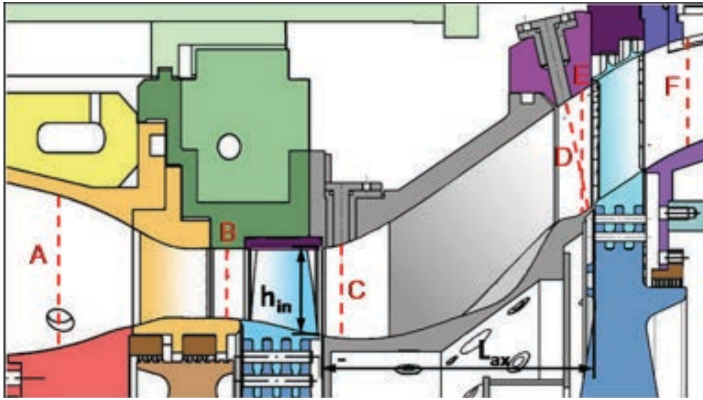
Figure 2. Meridional section of the test setup showing the HP stage between planes A and C, and the LP stage between C and F.
