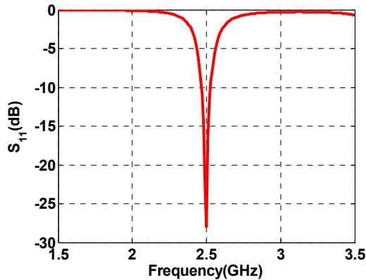
Fig. 3. Reflection coefficient of single patch antenna
