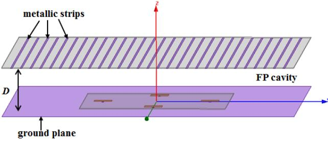
Fig. 6. Configuration of the OAM antenna & FP cavity
