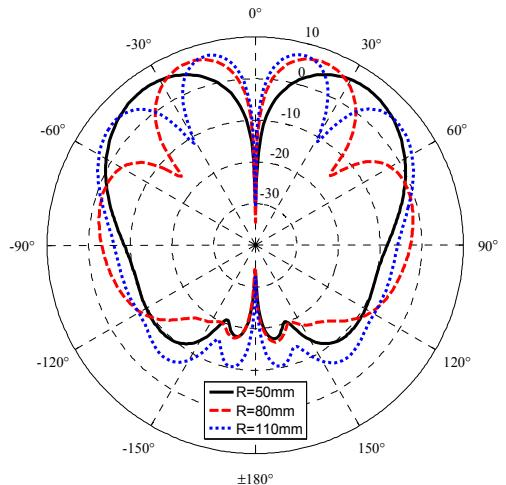
Fig. 5. E-plane radiation patterns with different array radiiuses
