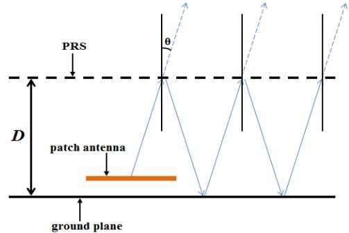
Fig. 1. Model of the FP cavity with PRS
