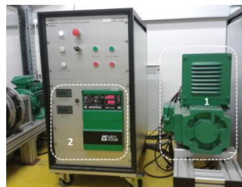
Fig. 3. An Induction machine used as a load.
