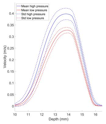
Fig. 2. Estimated velocity profiles on average (with all phantoms from 2 to 5 cycles) for the high pressure (blue) and the low pressure (red) at 333.33 ms.
