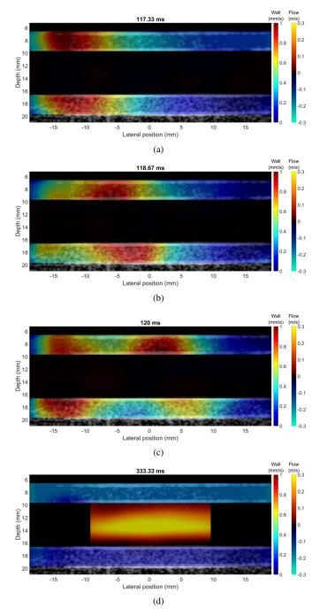
Fig. 1. Four snapshots of the wall and flow velocities at 117.33 ms (a), 118.67 ms (b), 120 ms (c) and 333.33 ms (d) after the beginning of an acquisition. Wall velocity is expressed in mm/s while flow velocity is displayed in m/s only on the center part of the lumen. (a), (b) and (c) show the pulse wave arriving from the left part of the phantom. (d) corresponds to the time when the flow is maximum at the center of the lumen.
