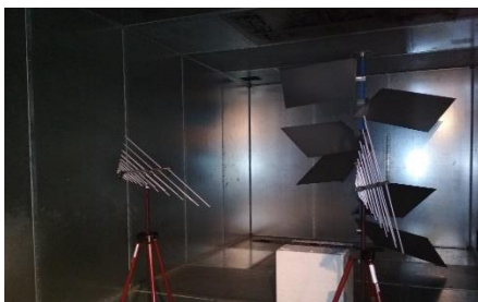
Fig. 2. IETR's reverberation chamber with the two log-periodic antennas and the three masts.
