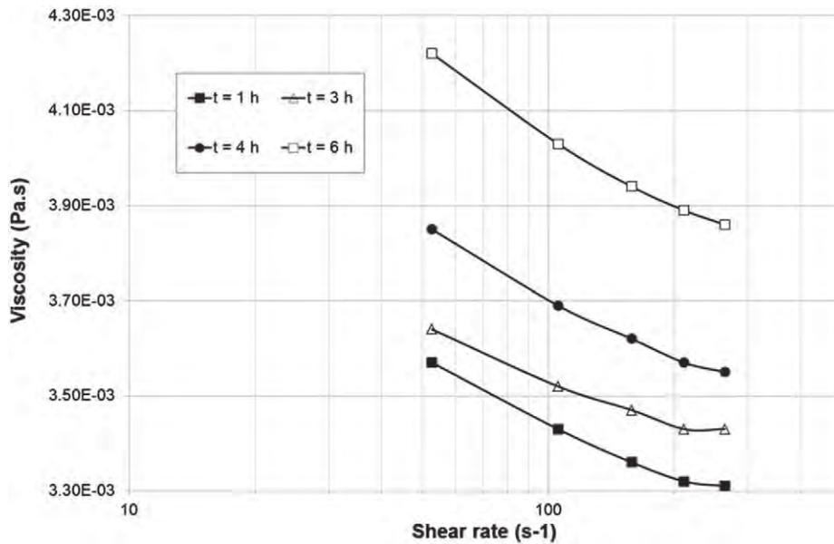
Fig. 7. Evolution of suspension viscosity ( $V_t = 5.7$  m/s,  $c_m = 0.3$ ) as function of shear rate for different grinding times.
