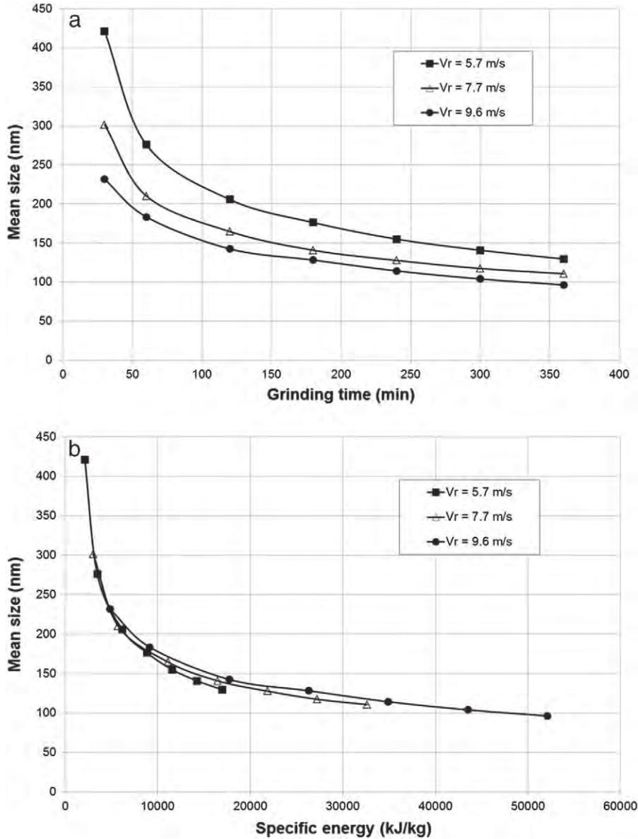
Fig. 3. Effect of stirrer tip speed on grinding result. a) Particle mean size versus grinding time. b) Particle mean size versus specific energy.
